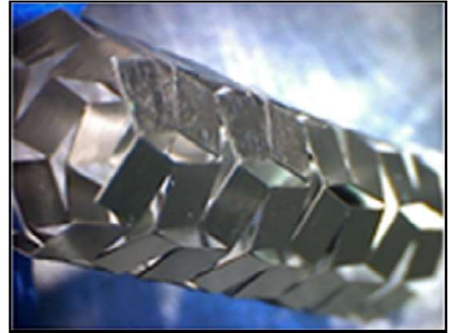
Fig: Polyurethane auxetic oesophageal stents Source: [2]
