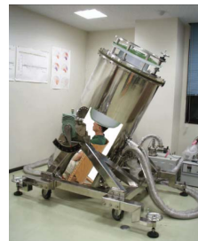
Superconductive Shielding : Shielding factor: 10 000 bei 0.05 Hz
