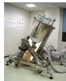
Superconductive Shielding : Shielding factor: 10 000 bei 0.05 Hz
