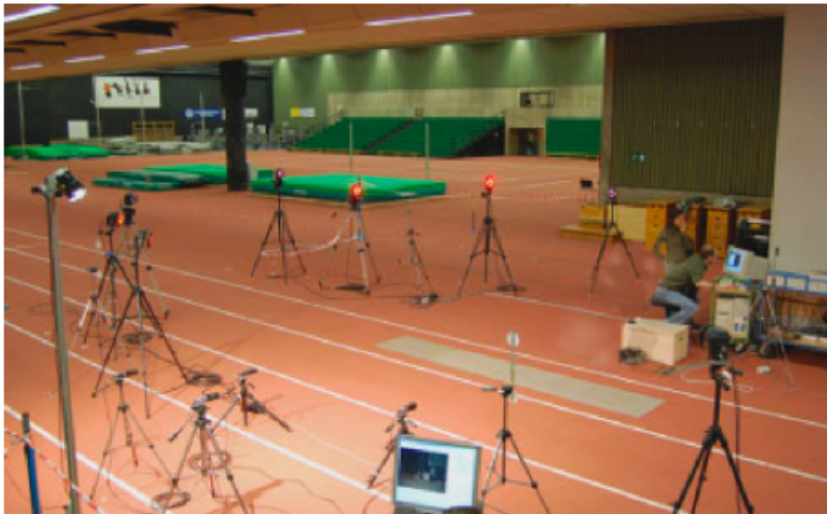
Figure 1. Experimental setup. Four force plates in series were embedded in the indoor track. Force plates were covered with the same material (different color) as the entire indoor track. Twelve Vicon cameras arranged around the force plates captured the athletes' motions.
