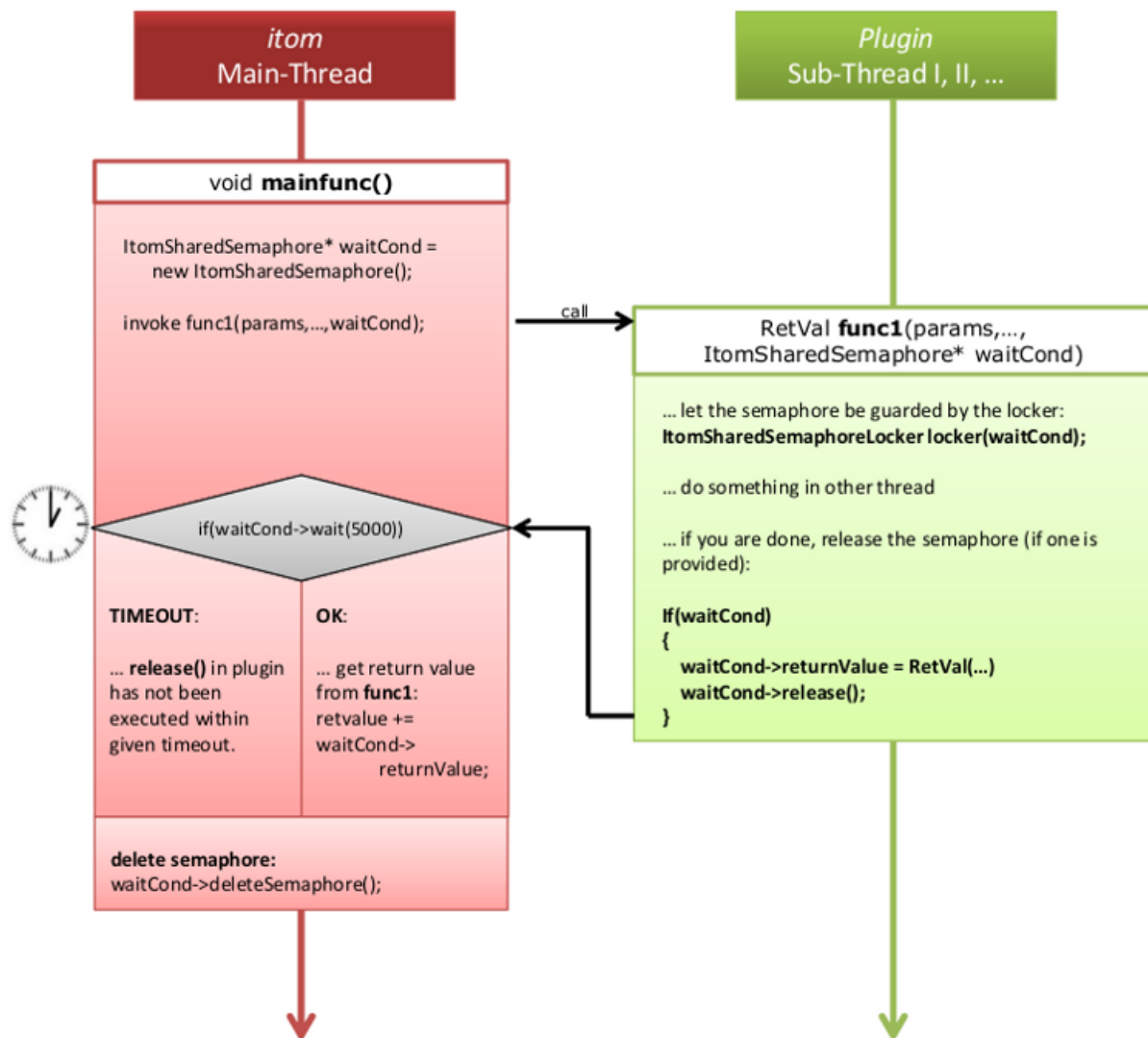
Figure 7.1: Figure: Scheme of a communication between itom (main thread) and any plugin-method (plugin is running in another thread)
