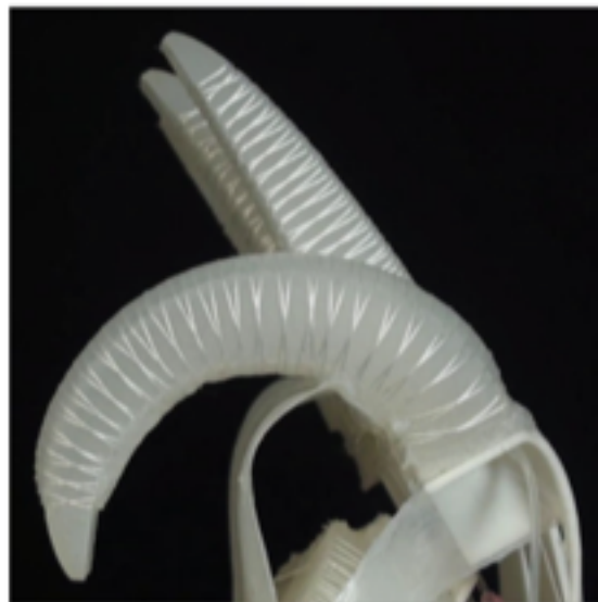
(a) An inflated PneuFlex actuator in front of deflated ones.
