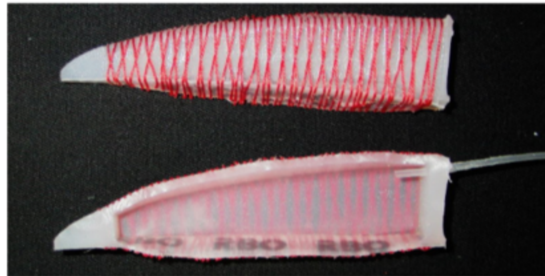
(b) Cut of a PneuFlex continuum actuator.
