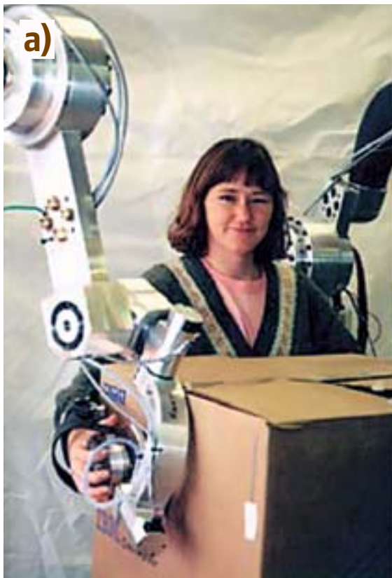
Fig. 33.3a,b Two-handed upper-extremity exoskeleton where artificially built friction forces between the load and the arms allow for grasping objects [33.25]
