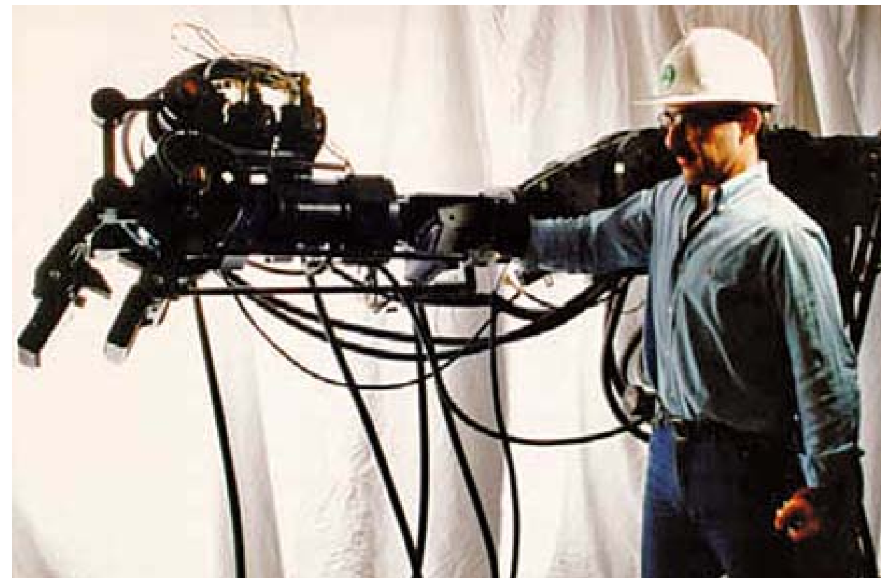
Fig. 33.4 One-handed upper-extremity exoskeleton where a griper allows for grasping of heavy objects [33.21]
