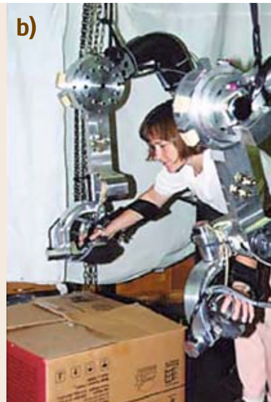
Fig. 33.3a,b Two-handed upper-extremity exoskeleton where artificially built friction forces between the load and the arms allow for grasping objects [33.25]
