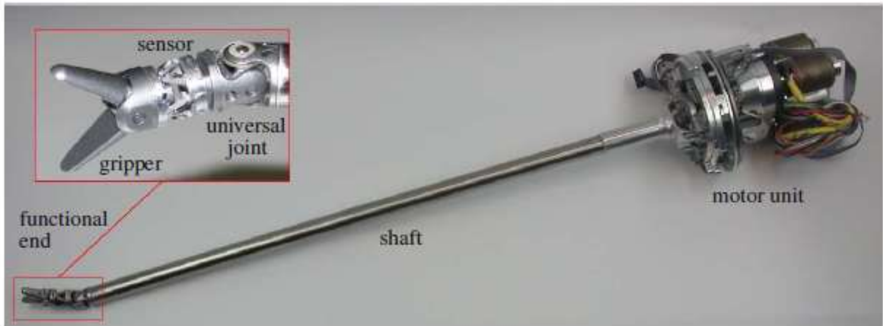
Fig. 1.3: Previous version of the DLR MIRS instrument. The gripper branches are developed in a basic form. In the instrument presented in this thesis the end-effector (gripper) is replaced by the ultrasound transducer, cf. Fig. 1.4 (photos: DLR).
